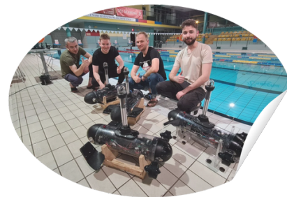
The CyberFish project is an underwater vehicle designed to mimic a fish, both in its external appearance and its movement.
